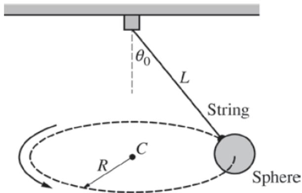
A small sphere of mass  $M$  is suspended by a string of length  $L$ . The sphere is made to move in a horizontal circle of radius  $R$  at a constant speed, as shown above. The center of the circle is labeled point  $C$ , and the string makes angle  $\theta_0$  with the vertical.
