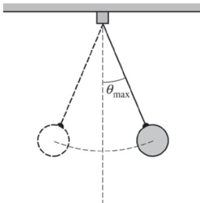
Instead of moving in a horizontal circle, the sphere now moves in a vertical plane so that it is a simple pendulum, as shown above. The maximum angle  $\theta_{max}$  that the string makes from the vertical can be assumed to be small. The graph below shows data for the square of the pendulum period  $T$  as a function of string length  $L$ .
